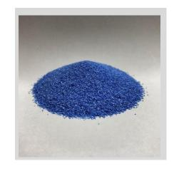
It is mainly used in deeply cutting, large feeding and forming grinding. In addition, compared with synthetic diamond and CBN, ceramic corundum abrasive has better versatility, which can be used for not only dry or wet grinding with water or oil cooling, but also for grinding black and non-ferrous metals, and effectively applied to grinding special materials such as stainless steel and heat-resistant alloy.
